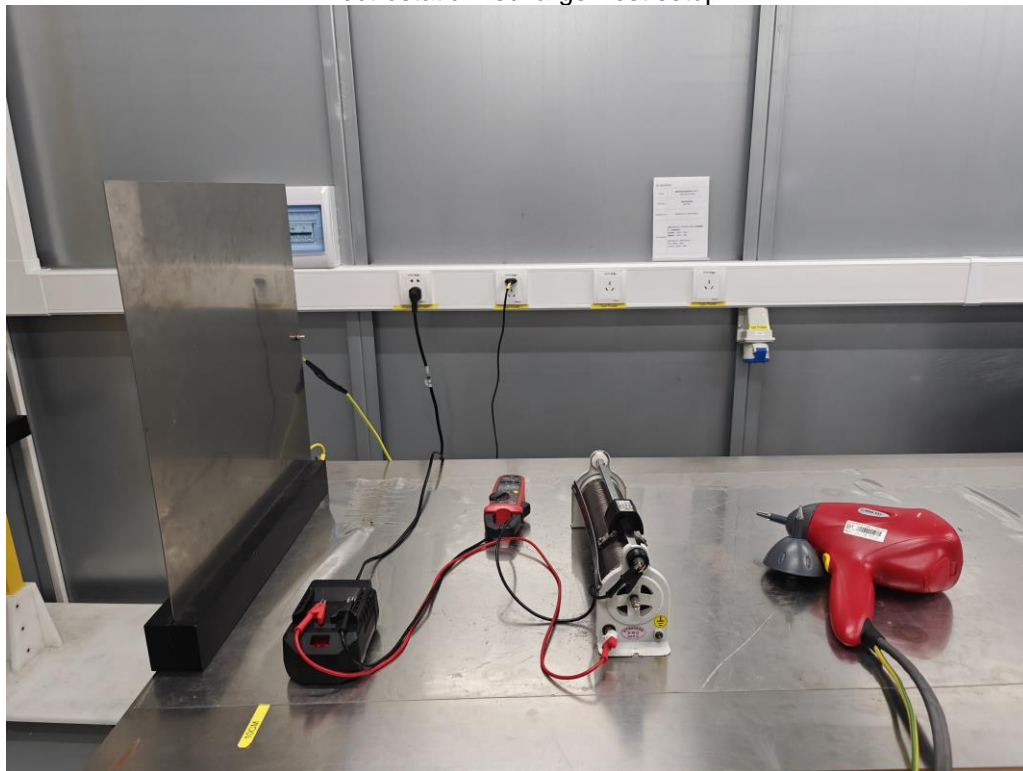
Electrostatic Discharge Test setup
