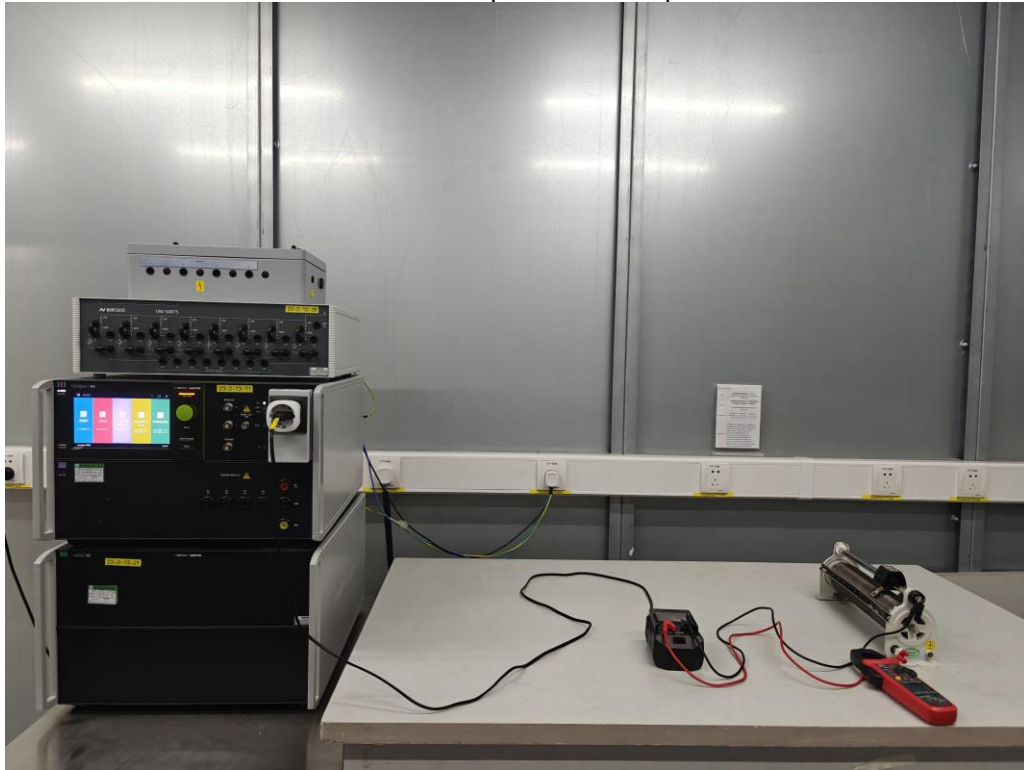
Injected Currents (RF common mode) Test setup
